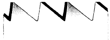
AMOUNT OF TOOTH FILED AWAY IN SECOND POSITION
